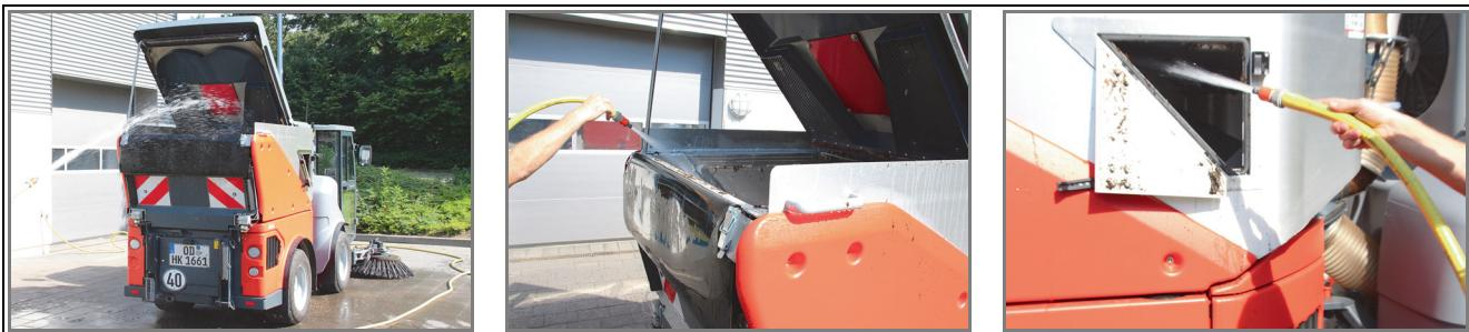
Raise the dirt hopper approx. 50 % so that the water and dirt can be tipped out. Clean the entire dirt hopper from the inside.
